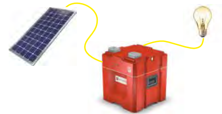
Standalone Power-Blox Instant plug & power Directly supplies 230 V AC
